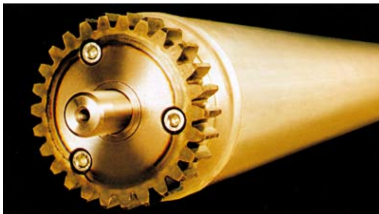
Euro cloth beam with guide slot and gear on one side
