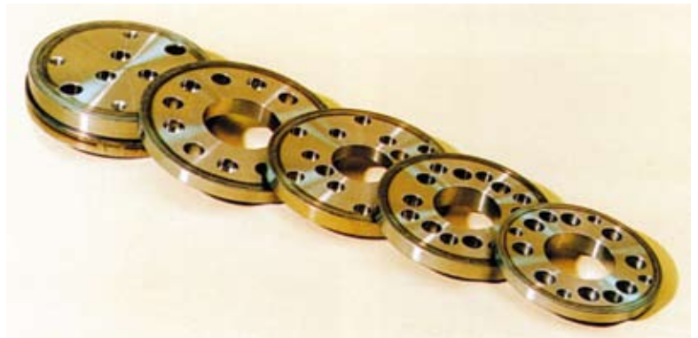
Bearing ring for fixed flanges, turned, drilled, hardened, ground, phosphatized for all loom types in question
